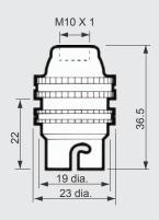
**GP-015**: B-15 Brass Lampholder, 10mm or  $\frac{1}{2}$ " entry thread, with shade ring and earth tag.
